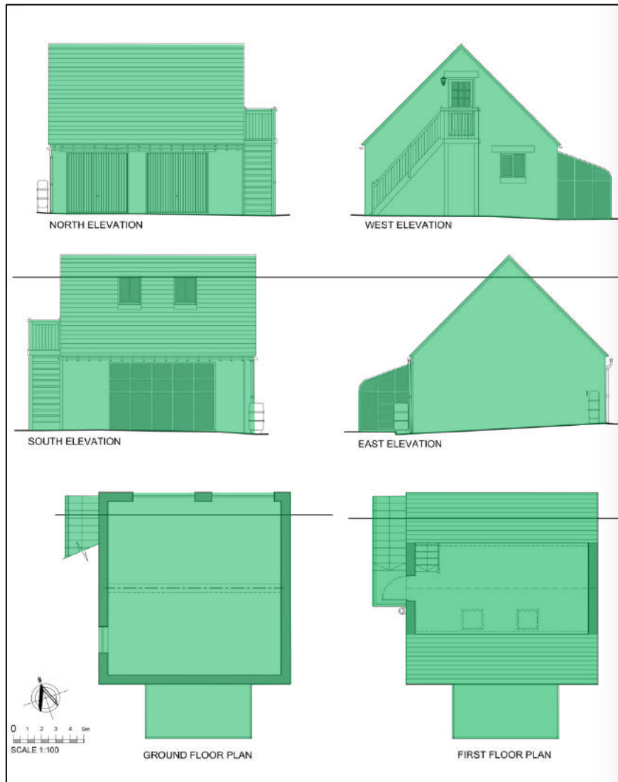
Existing floor-plans (prior to any conversion), 17/03060/FUL. Existing building shaded green for clarity.
